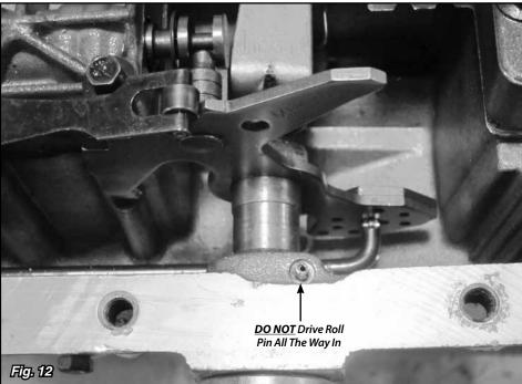
With OE Column (Rod Type) Linkage or Lokar Cable Type Linkage, Put Trans Arm at 7:30 Position in "PARK"
