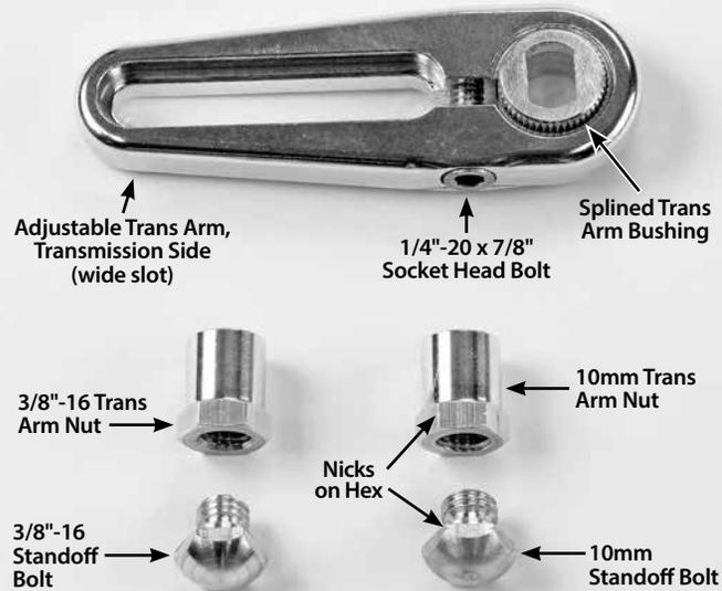
Standoff Bolt is only used with the Lokar Backup Light Switch or Neutral Safety Switch (not included).
