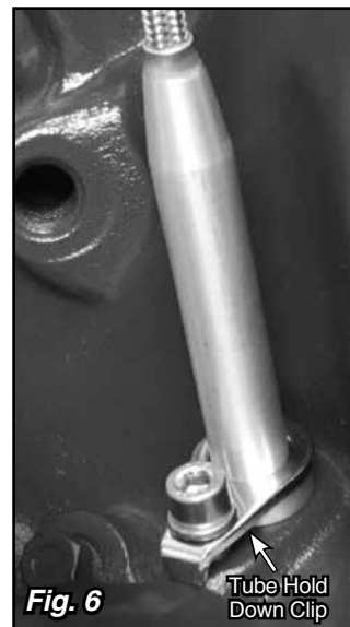
Kickdown Kit shown installed with Lokar Throttle Cable (not included) and Lokar Double Stud Tuned-Port Bracket (not included).
